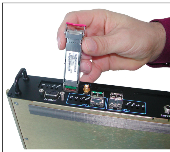
Fig.3: Change the optical interface of your module in the field via XFP/SFP transceivers
